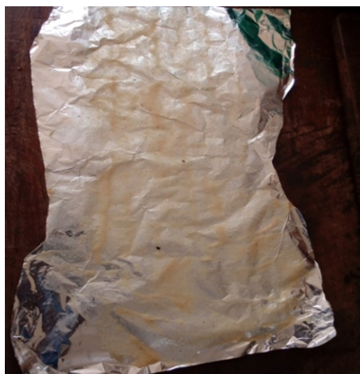
Figure 3: Starch paste on aluminum foil for drying
