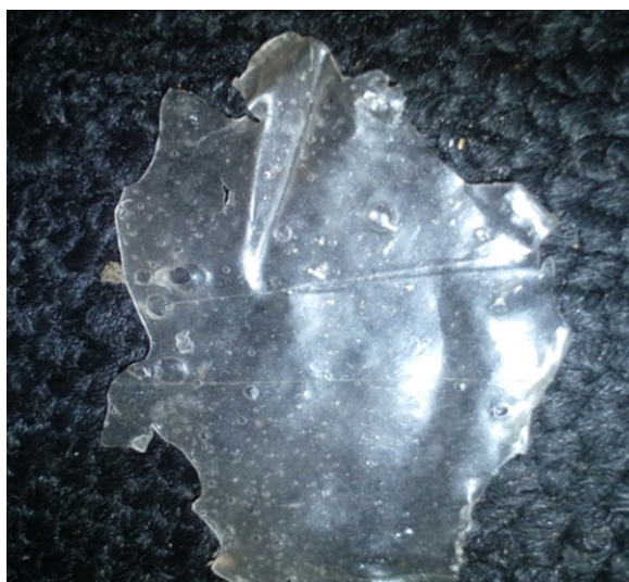
Figure 4: Bioplastic film after drying
